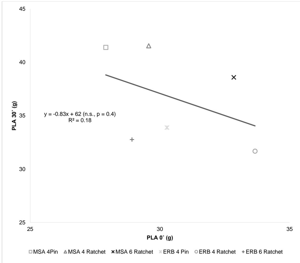
Figure 10 - Correlation between PLA measurements for forward-flexed head posture versus upright head posture for a steel impactor
