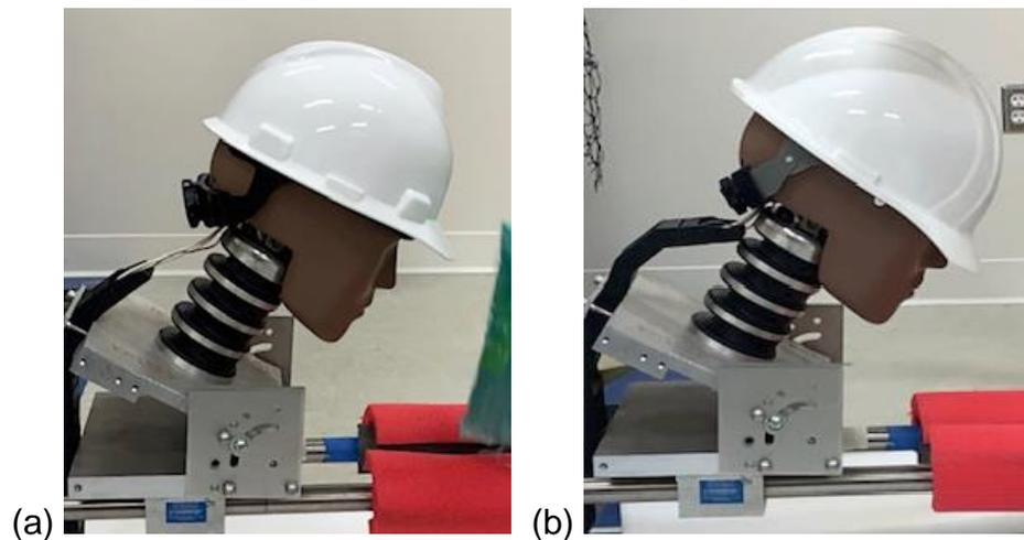
*Figure 11 - Still frames taken from high-speed video showing (a) an MSA hard hat and (b) an ERB hard hat immediately post impact.*
