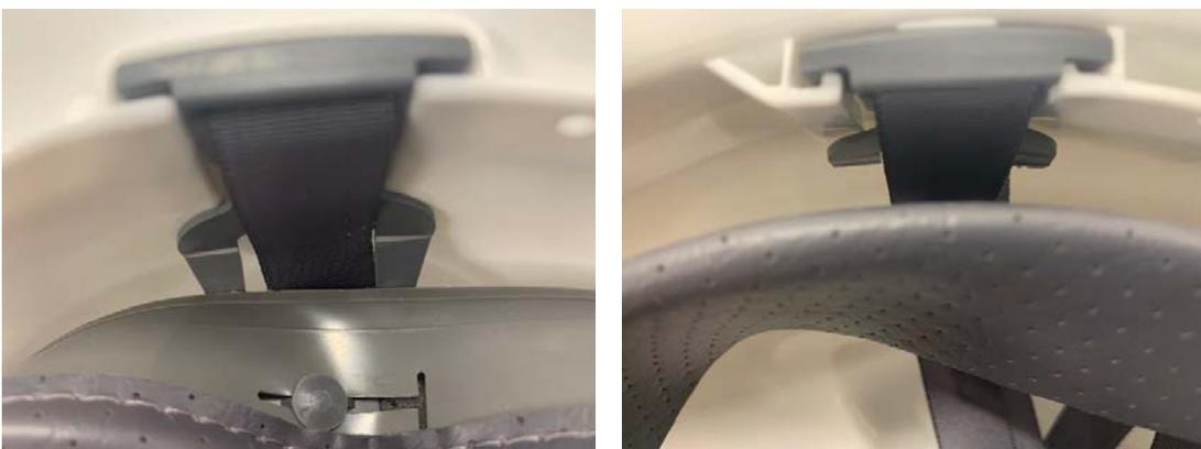
*Figure 7 - Undamaged MSA plastic attachments (left), damaged MSA plastic attachments (right)*
