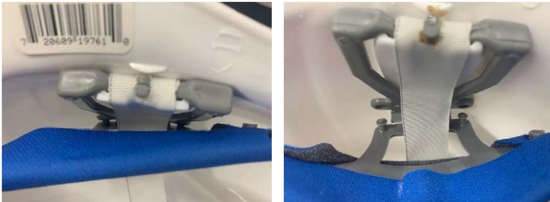
*Figure 6 - Undamaged ERB plastic attachments (left), damaged ERB plastic attachments (right)*
