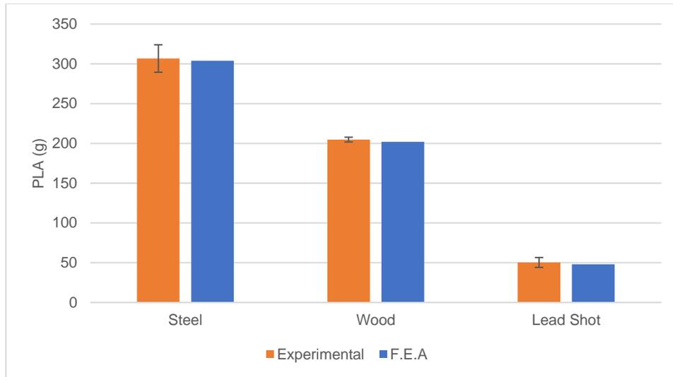
*Figure 16 - PLA for unprotected tests, used in calibration/validation of impactor material properties*
