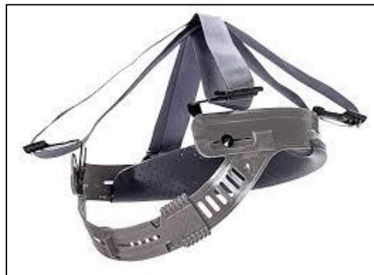
*Figure 12 - Example of a hard hat headband and nylon suspension system. Note that the headband connects to the shell via the four hinged polymer structures, which have been flipped out to horizontal position for visibility<sup>56</sup>*
