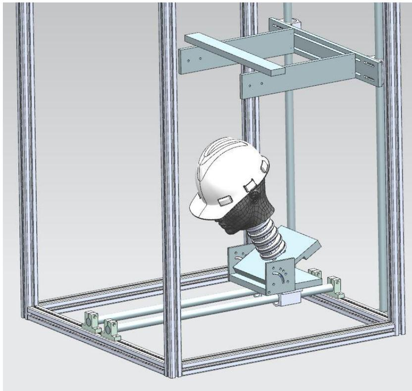
*Figure 8 - Rendering of the drop rig fixture used in experiments, showing the head in a forward-flexed position prior to impact.*
