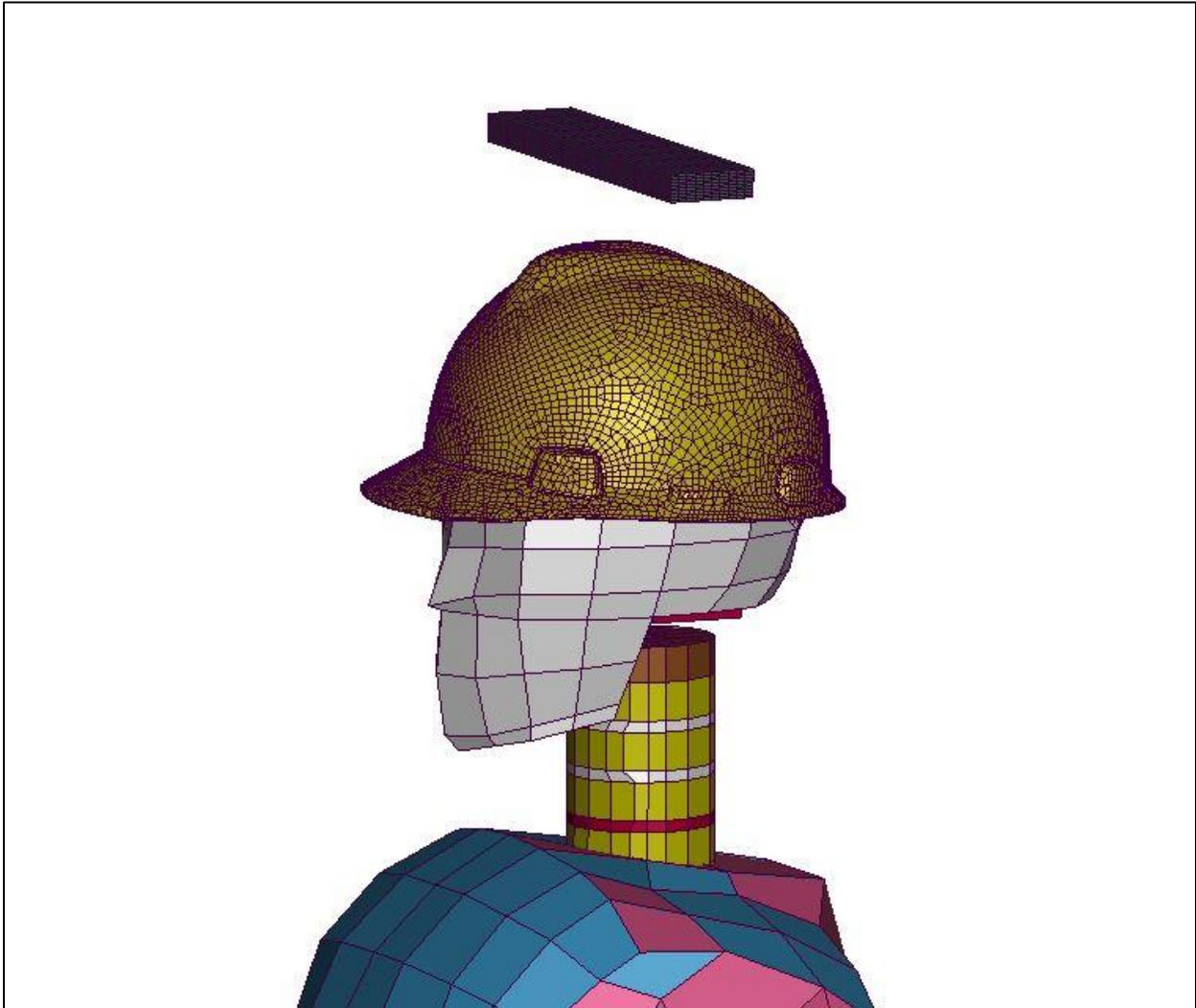
*Figure 15 - Finite Element Simulations Test Configuration*
