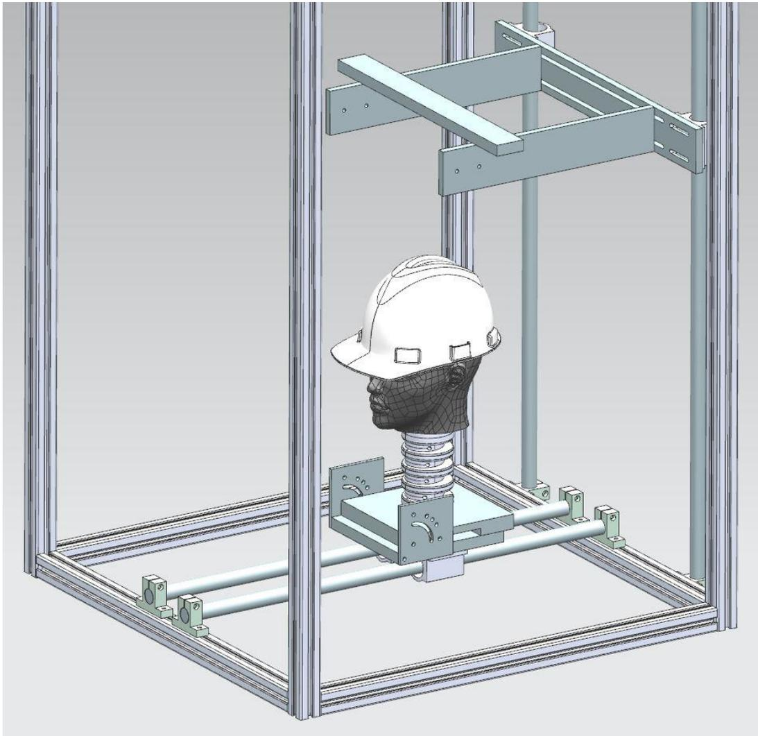
*Figure 4 – Rendering of drop rig test fixture*
