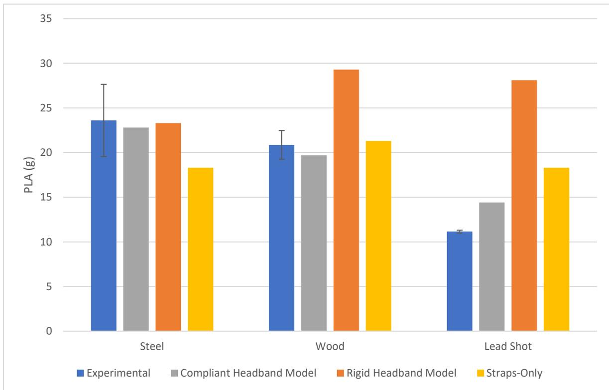
Figure 17 - Summary of the PLA Results Obtained by Each Hard Hat Model in Comparison to Experimental Testing
